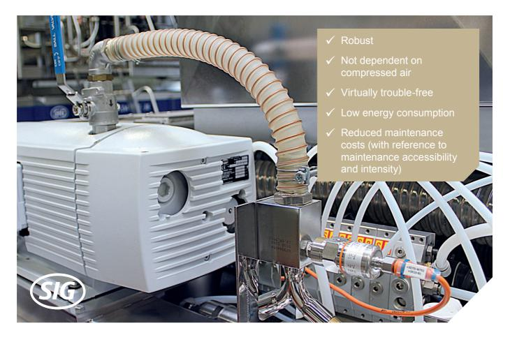
The function of a vacuum pump in the folding zone can be quickly explained: It creates negative pressure via a vacuum in the suction bar, so that the carton is removed from the magazine by means of small suction cups and then placed in such a way that it can be picked up by the mandrel wheel. That means the vacuum pump is partly responsible for transporting the carton – and right at the sharp end too.
